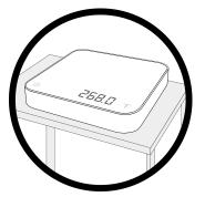
Select a work place that is stable, vibration-free and, if possible, a horizontal location for the weighing platform.
