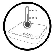
• Avoid places where room temperatures are unstable. Room temperature above 40°C or below 15°C may result in weighing inaccuracy.
