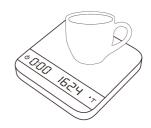
The timer starts when the flow of espresso is detected.
