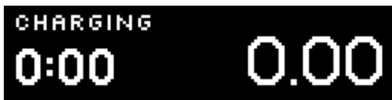
When connected to a USB Type-C charger while the Pyxis Black is on, the word **CHARGING** will appear in the top-left corner of the display.
