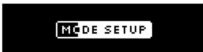
The Tare Button provides quick access to mode settings. Press and hold the button for about 1 second until the display shows **MODE SETUP**, then release it to open the menu.
