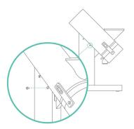
2 Remove the M3x8 mm screw on the left side of the motor housing of the Orbit.
