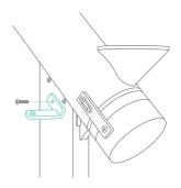
Align the short side of the L-Shaped mount with the Orbitand secure it in place with an M3x12 mm screw as shown. Ensure the long side of the mount is perpendicular to the Orbit housing.
