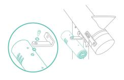
4 When installing the Ion Beam, place a spacer on both sides ofthe screw hole of the L-shaped mount, then secure it with a 1/4-20x12 thumb screw. After installing the Ion Beam, adjust its position to a 45-degree angle toward the chute.
