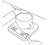
2 Place a cup on the scale and tare the weight manually.
