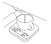
3 The timer starts when the flow of espresso is detected.
