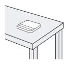
Place the scale on a stable and vibration-free surface at a preferably horizontal location.
