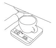
4 The timer will stop automatically when the espresso flow stops or the cup is removed.
