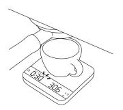
1 The timer will stop automatically when the espresso flow stops or the cup is removed.
