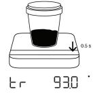
2 Press and hold Tare button for 0.5 second. The scale will display the weight to be deducted.
