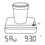
Press and hold Tare button for 2 seconds when reading is stable. The weight is stored as a preset container weight.
