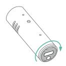
5 Reattach the front cover carefully, ensuring it is securely fastened to maintain proper functionality.
