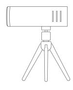
1 Insert the tripod screw thread into the designated tripod socket on the Ion Beam. A standard 1/4- inch tripod socket ensures universal compatibility.
