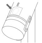
Remove the original hopper. Cover the bean chamber with the sticker inside the package. The sticker prevents screws from falling into the bean chamber.
