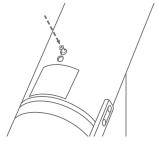
Secure the screw in the upper hole using a #1 PH screwdriver.
