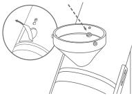
Remove the sticker and attach the Multi-Purpose Hopper to the grinder with a #2 PH screwdriver.
