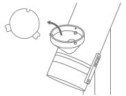
Ensure the hopper is fastened firmly to the grinder. Once secure, remove the paper blocker from inside the hopper.
